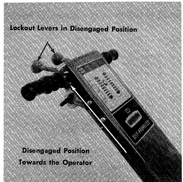
FIGURE 22. LOCKOUT LEVERS DISENGAGED
